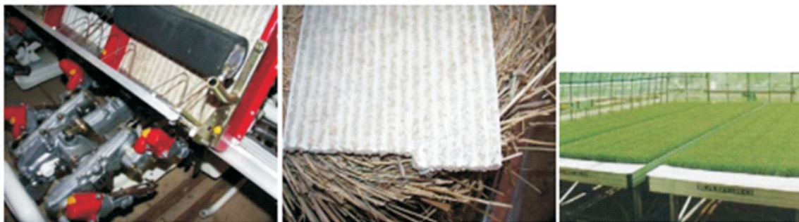
Figure 1. (Left) Japanese transplanter adapted to take a seed mat, (Centre) Seed mat with rice seeds and fertiliser embedded in card (Right) Rice seedlings ready for transplanting
